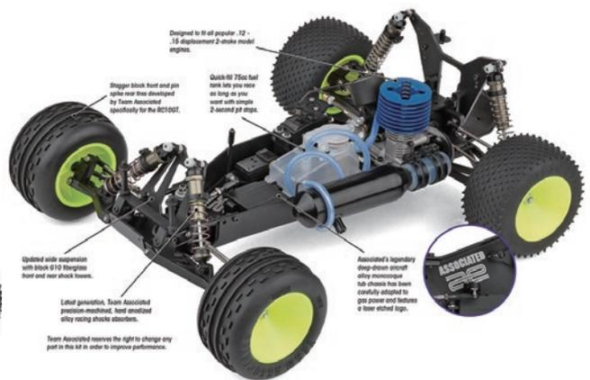
Designed to fit all popular 12 - 15 displacement 2-stroke model engines.
